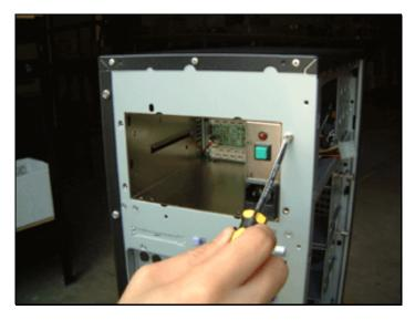
Install redundant power supply's housing and secure it with screws
