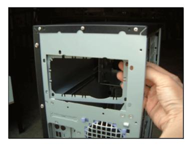
Remove the power supply bracket.
