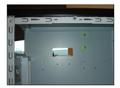
Remove two posts (circled in green on the image) inside the case if necessary.
