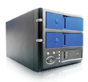
v7AGE220-SAU is for use with two 3.5" SATA II hard drives. The storage capacity of the hard drive is unlimited. It has screw-less design for easy installation. 2 LEDs for power on and HDD activity and 6 blue LEDs for RAID level and data connection. It has internal power supply.
