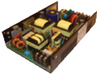
CP-M0402DU Series (U-Chassis Type): 8(L) x 5(W) x 1.6(H) inches.
